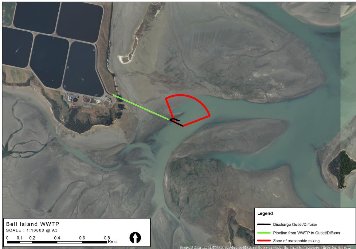
Figure 1. Zone of reasonable mixing, being defined as the area delineated by a 250 metres radius north of the outfall and within 45° included angles.
